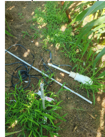
... a ~2400 € probe smashed by a tractor (top) or animal (bottom)
